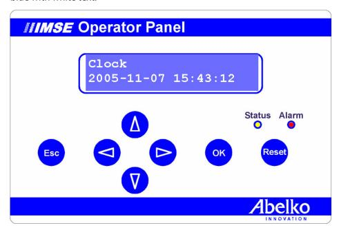
The panel has seven keys, an alarm LED and a status LED. It uses a 12 V power supply, which can be taken from the WMPro, and is connected to the RS485 A and B terminals.
